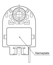
When a positive electrode (+) is connected to the Red lead wire, and a negative (-) electrode to the Black lead wire, the shaft rotates clockwise (in the direction shown by the arrow).
